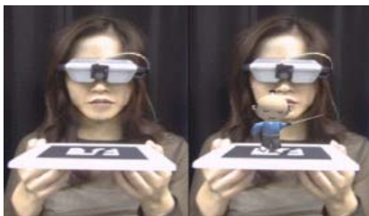
Figure 1. Augmentation based on 2D pattern (left figure contains a 2D pattern, and that of the right shows the scene after augmentation) [3]
